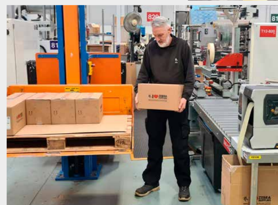
← Photo 4 Lifts box and turns to place onto pallet at same height as packing line
