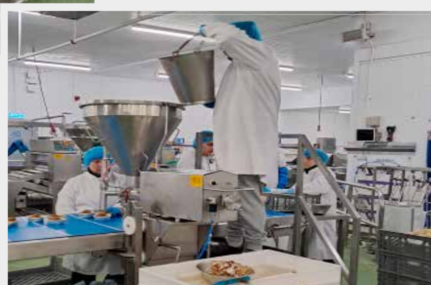
← Photo 1 The operator bends down to scoop the pie fill from the tote bin into a small bowl before decanting it into the transfer bucket
