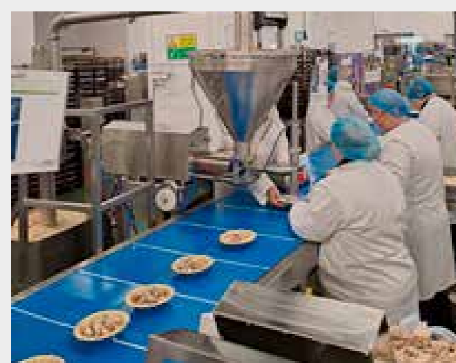
→ Photo 3 The hopper topper transfers the pie fill from a tote bin into the hopper to eliminate MSD risk
