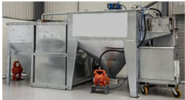
**Figure 15** Waste water/slurry management system
