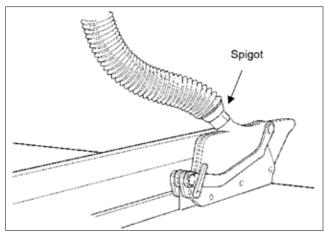
Figure 1 Improving volume flow rate on crown guards
