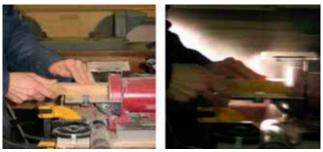
Figure 3 Effectiveness of a dust lamp in showing the dust cloud produced by sanding. This is normally invisible to the naked eye
